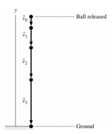
Assess: The average velocity keeps increasing with time since the ball is speeding up as it falls.
