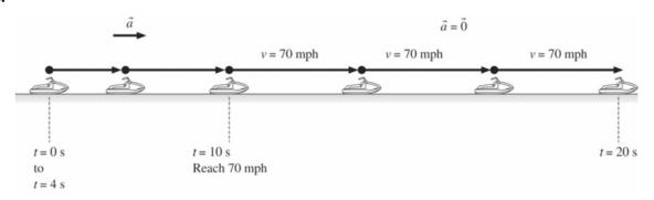
Assess: Notice that the acceleration vector points in the same direction as the velocity vector because the jet ski is speeding up.
