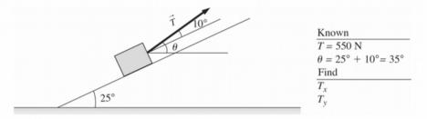
**Solve:** First find the angle from the horizontal:  $\theta = 25^{\circ} + 10^{\circ} = 35^{\circ}$ .
