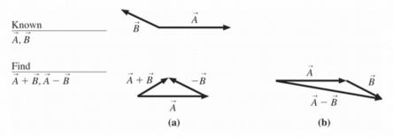
**Solve:** (a) To find  $\vec{A} + \vec{B}$ , we place the tail of vector  $\vec{B}$  on the tip of vector  $\vec{A}$  and draw an arrow from the tail of vector  $\vec{A}$  to the tip of vector  $\vec{B}$ .
