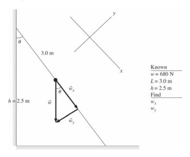
**Solve:** First find the angle of the ladder from the vertical:  $\theta = \cos^{-1} \left( \frac{2.5 \text{ m}}{3.0 \text{ m}} \right) = 33.56^{\circ}$ .
